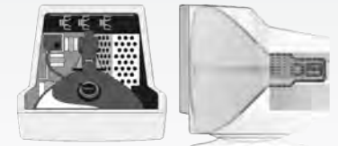
illustration of a cathode ray tube (CRT) inside a computer monitor
